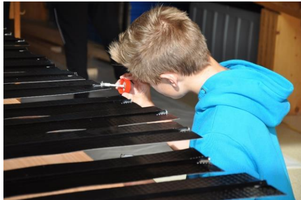
Applying the solder paste to the absorber tubes
