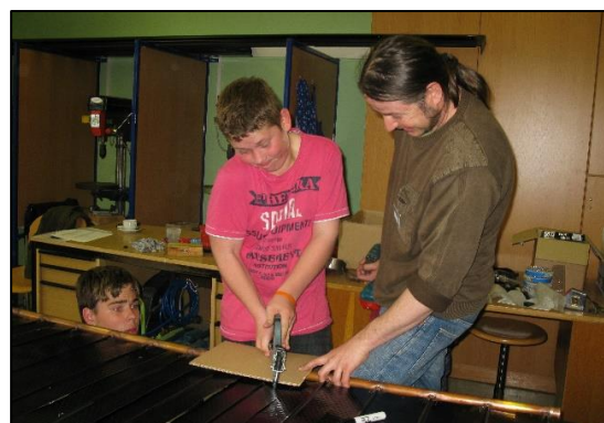
8. Fixing of the absorber strips with rivets
