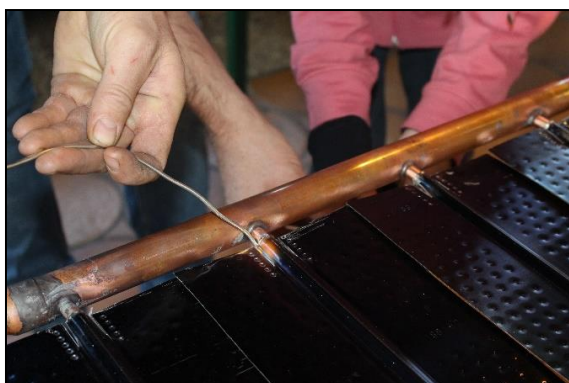
7. Attaching and soldering the copper manifolds to the absorber strips
